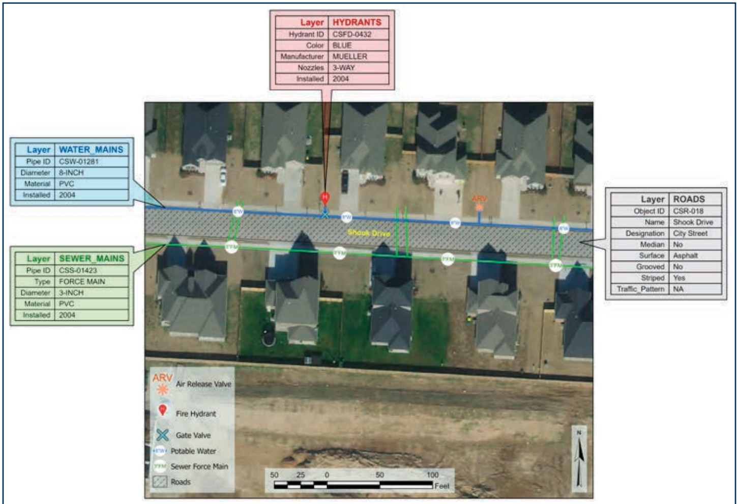
A GIS map of municipal utilities may include not only where the service lines are located, but layers of other relevant information as well.
